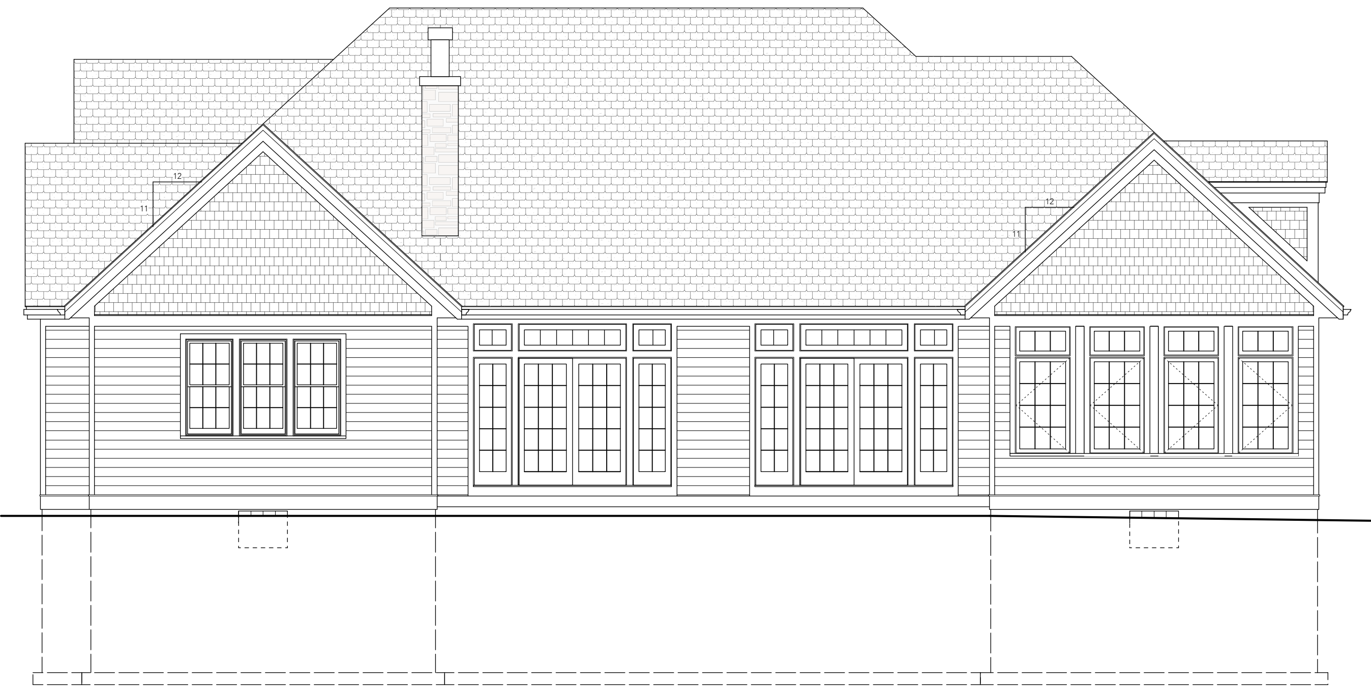
2 EXISTING/DEMOLITION REAR/SOUTH EXTERIOR ELEVATION D201 Scale: 3/16" = 1'-0" 01'-0" 5'-0" NO WORK PROPOSED FOR SOUTH ELEVATION
